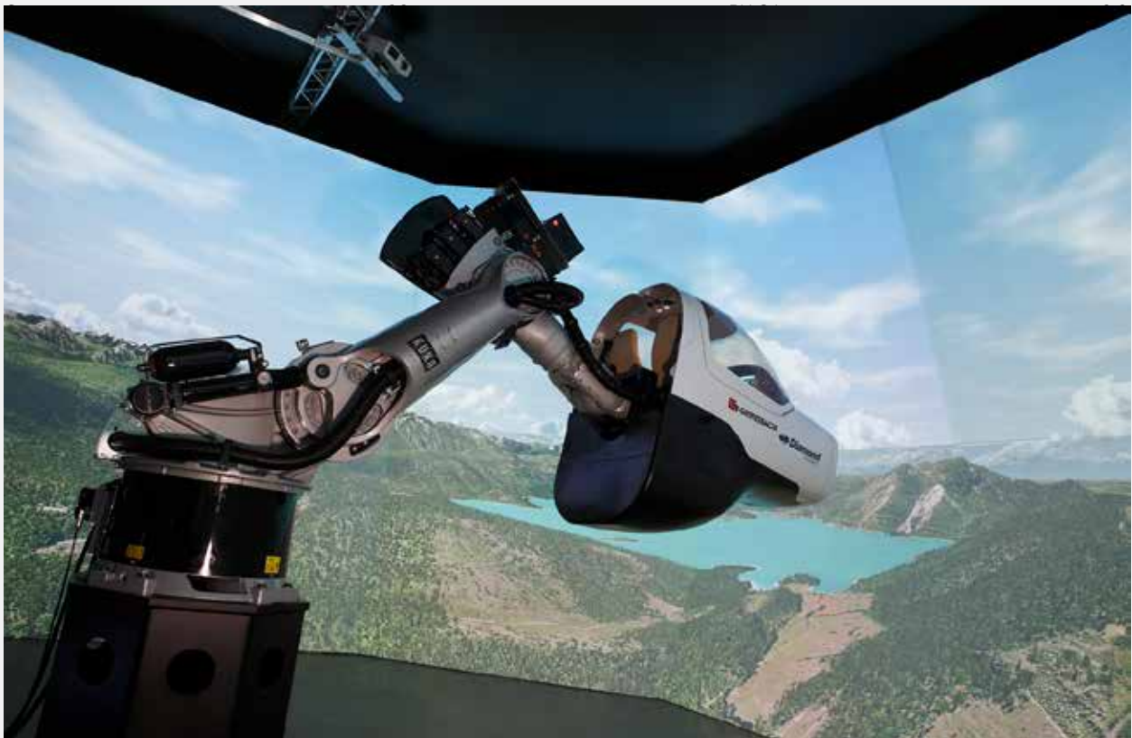
Figure 5: CAVE as Rear Projection-based Virtual Reality Display
